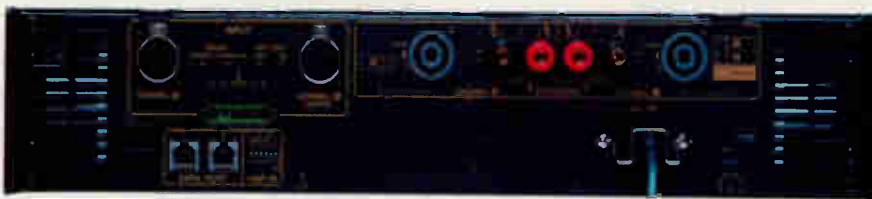
Yamaha PC9501N's rear panel features balanced XLR and Euroblock connectors.
