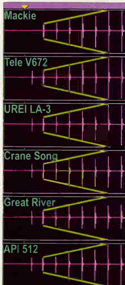
Figure 2: Successively louder snare hits, as captured by six preamps. Note how a purposely overloaded preamp levels the transients like a peak limiter.
