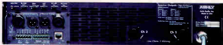
Ashly Audio Protea Enabled Series 3800 can be controlled/monitored via built-in Ethernet.
