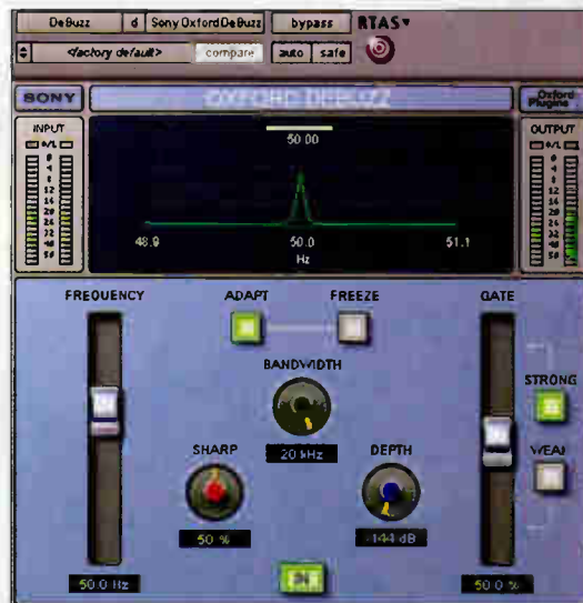
DeBuzz controls frequency tracking with Adapt and Freeze settings.
