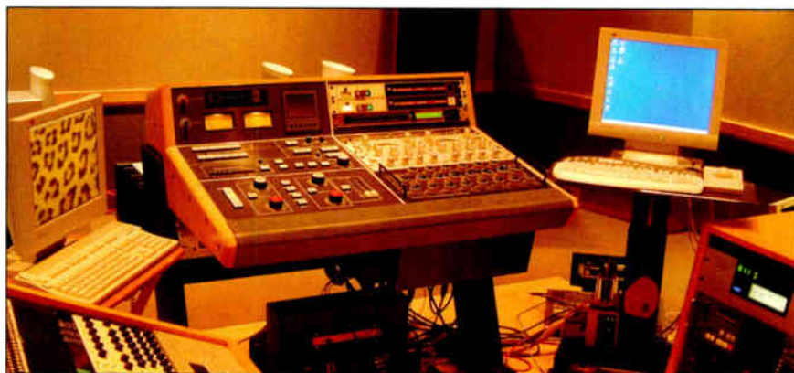
Album remastering guru (Grammys for The Complete Hank Williams and Martin Scorsese Presents the Blues, as well as surround work for Alicia Keys, Luther Vandross, G3 and Chevelle) Joseph M. Palmaccio's suite is outfitted with a David Smith custom analog board, numerous pieces of both analog and digital processing, a Sequoia DAW, an Ampex ATR-102 and Dunlavy speakers with Classe amps.
