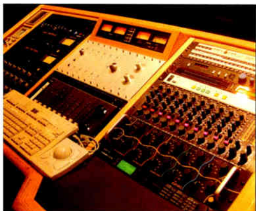
Three-time Grammy winner—who has mastered LPs for James Brown, Hank Williams and Parliament Funkadelic and SACDs for Norah Jones and Miles Davis—Mark Wilder relies on an SPL-proprietary console. Other gear of note includes Mastering Lab tube line amps, ATR-102 2-track with tube option and Dun-tech Princess monitors with Spectral amplification.
