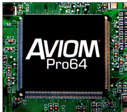
Aviom's custom Pro64 ASIC provides the core of the A-Net Pro network protocol, handling up to 128 channels.
