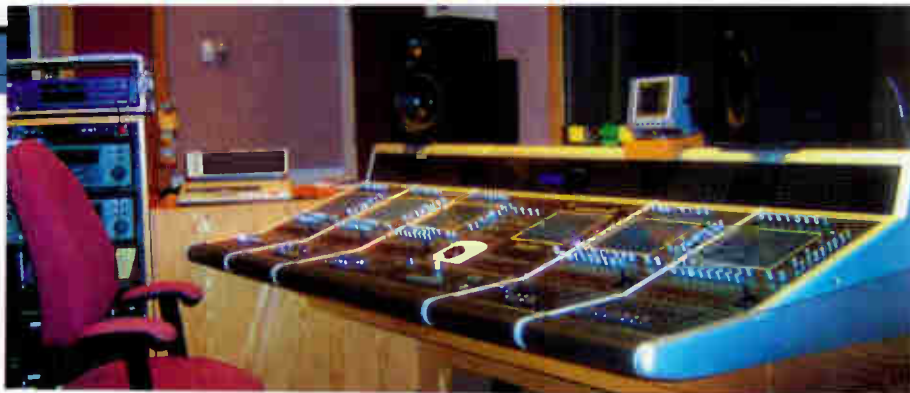
One of several Soundtracs digital consoles in use by the CBC, this DS-00 at CBC Radio in St. John's, Newfoundland, is used for music and drama production, and TV post work.
