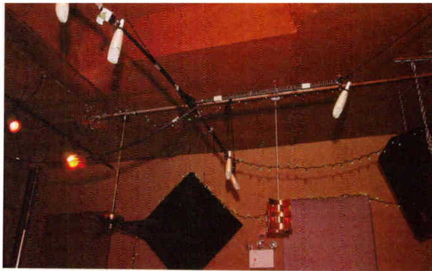
A view from the stage, looking up: The Decca Tree setup comprises three Shure KSM32s facing the stage and two facing the back to capture the room and audience.
