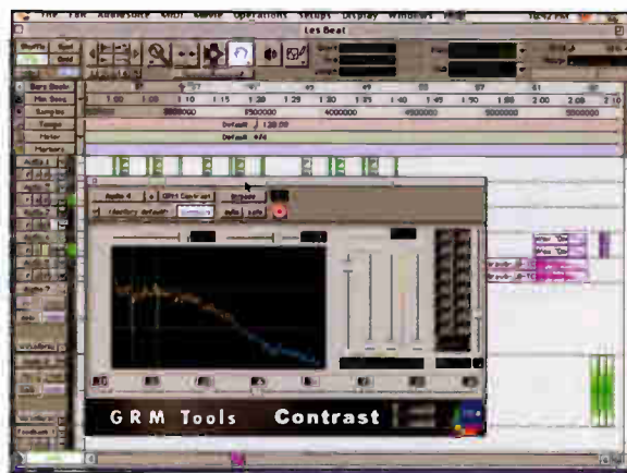
The Contrast plug-in, from the GRM Tools ST bundle, allows you to pinpoint weak parts of an audio file's frequency spectrum and bring them into the foreground.
