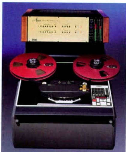
Ampex ATR-102 tape machine upgraded to be a 1-inch/2-track
