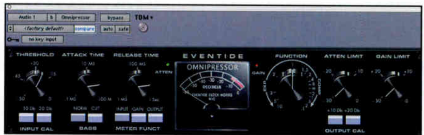
The Omnipressor plug-in offers Threshold, Attack and Release controls, as well as unique Function, Atten Limit and Gain Limit functions.
