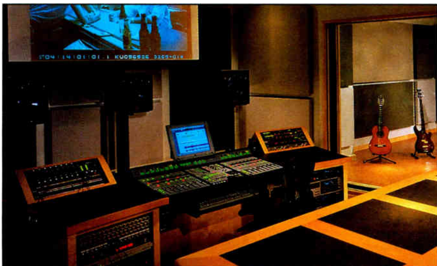
The console-less studio: The Mix2Pix Suite at Cincinnati's Sonic Arts Digital Audio Services features Digidesign Pro Control controllers with its Pro Tools systems, rather than a traditional console.
