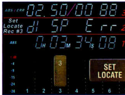
Figure 4: Three steps to access error rate on an ADAT: 1) the normal display, 2) the brief display that pops up after pressing Set Locate and Record Enable for track 3, and 3) the actual error rate display and condensed tape counter.
