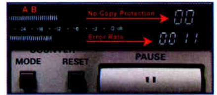
Figure 5: Press Mode-Reset-Pause simultaneously on a Panasonic DAT, then press Mode until the "AB" appears. Copy protection is also indicated in this mode.
