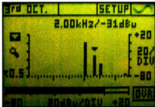
Even-order harmonics are generated by asymmetrical distortion as is common for some vacuum tube circuits. The cursor is over the second harmonic.
