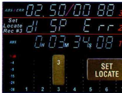
Figure 4: Three steps to access error rate on an ADAT: 1) the normal display, 2) the brief display that pops up after pressing Set Locate and Record Enable for track 3, and 3) the actual error rate display and condensed tape counter.
