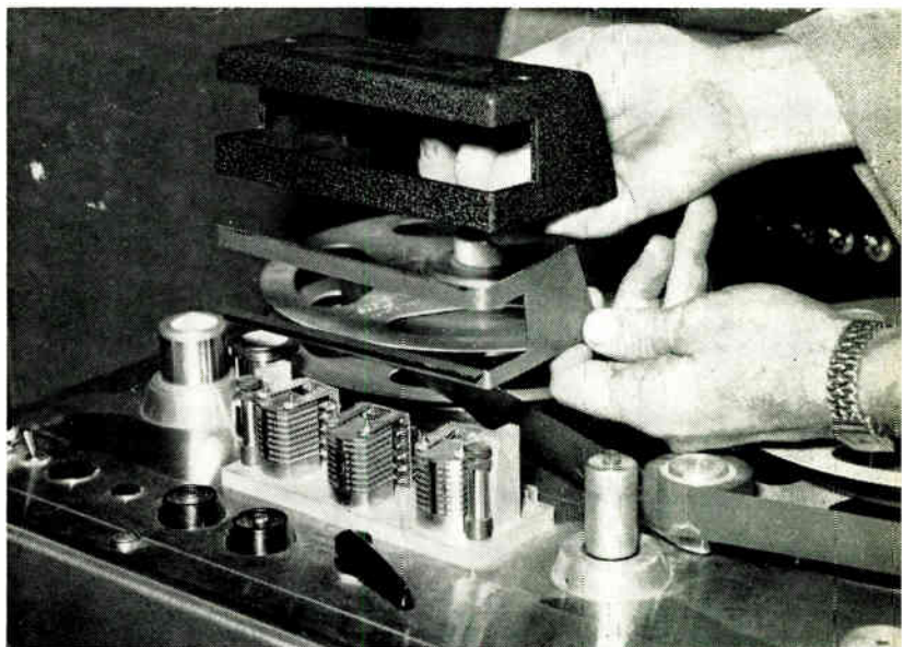
Fig. 5. Stacked heads assure perfect synchronization of all the eight channels
