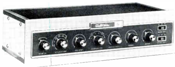
Fig. 4. Preamp provides all controls and switching for audio system
