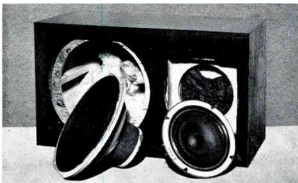
Below: Cabinet is partly filled with sound-absorbing material. Special 12-in. acoustic-suspension speaker, left, has 3.3-lb. Alnico 5 magnet. Smaller speaker is an Altec 755-A. Right: Field test of free-space response at low frequencies
