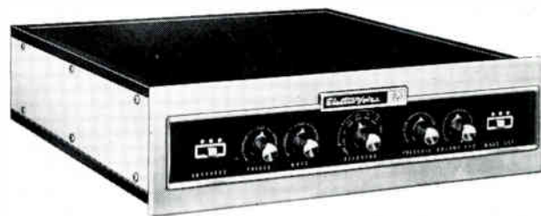
Fig. 5. Preamp and audio control center, with a 20-watt amplifier
