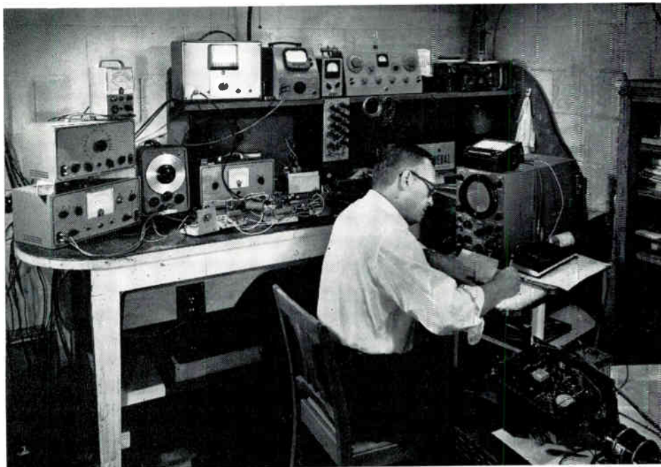
Closeup of the cutting equipment shown at the top of this page. Here is a rebuilt lathe, with a preamp, control box, and vacuum-tube voltmeter of Nunn's own design
