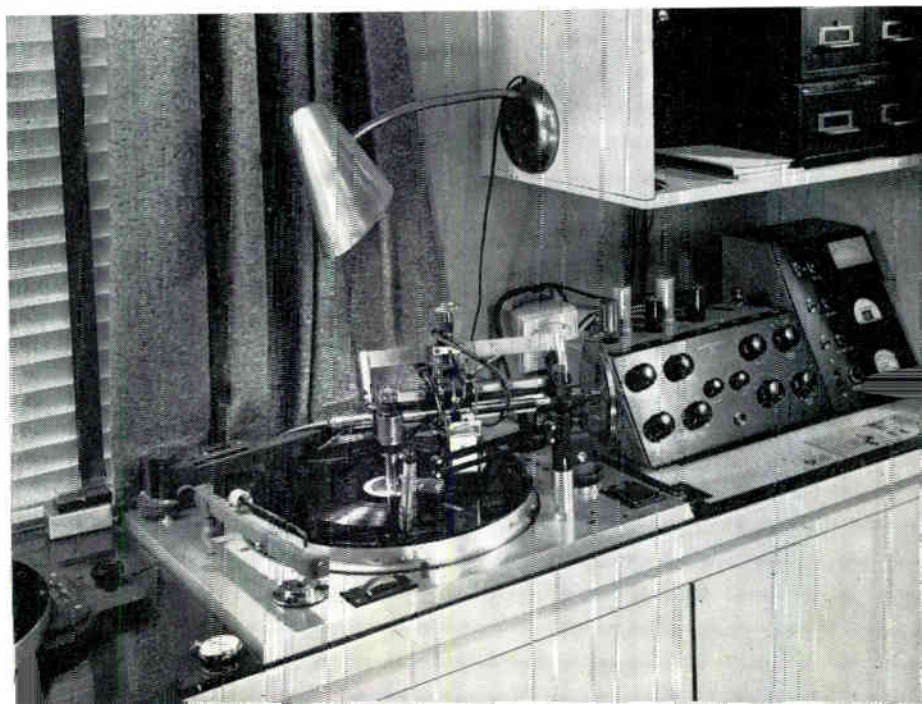
Closeup of the cutting equipment shown at the top of this page. Here is a rebuilt lathe, with a preamp, control box, and vacuum-tube voltmeter of Nunn's own design
