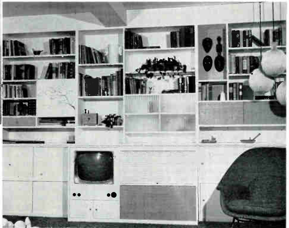
Below: a storage wall installation designed by George Orban for M. Alden Porter's apartment at Peter Cooper Village, New York City. Audio units are at the right of the TV tube, with all electrical outlets behind two small doors beneath. Records are stored behind sliding doors at left and right. Coaxial speaker is mounted behind pandanus cloth grille under the audio section. Woodwork is painted white to match the walls. See detail below
