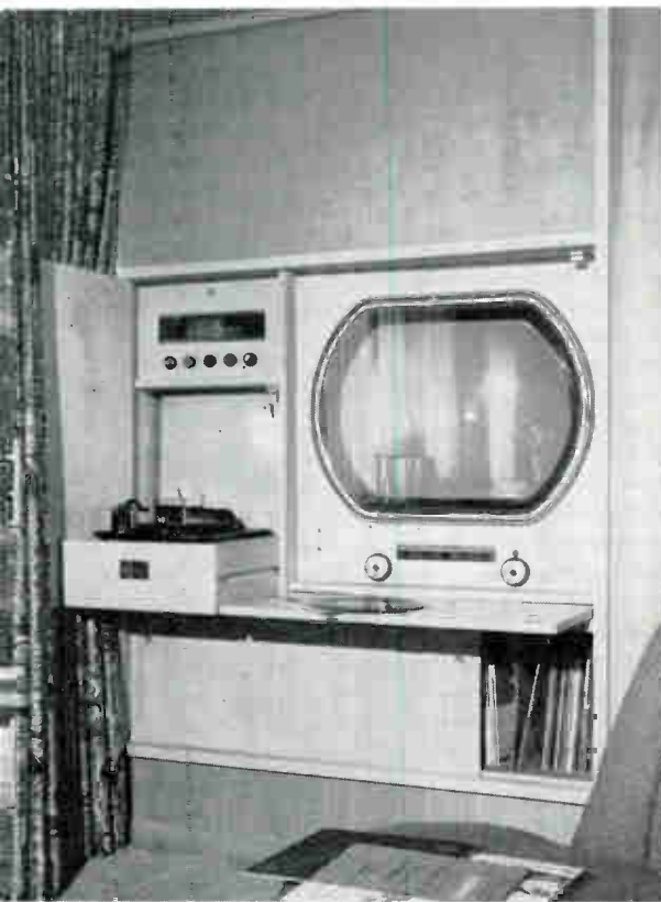
Above: Robert N. Marion, of Seattle, built this flush-wall installation in a closet. Door at left closes over the equipment, and pull-out shelf goes up to cover TV tube. Jacks at left of the TV tube are for connecting a recorder. Top section houses a bass reflex speaker; record storage at the bottom has two sliding doors
