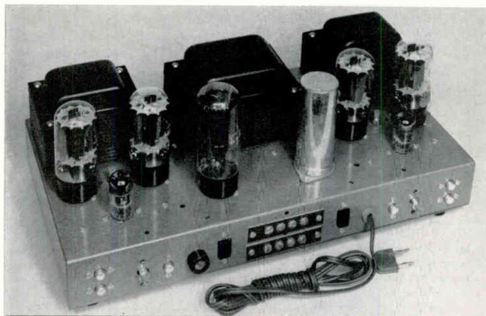
Fig. 4. Frontside of the Arkay stereo amplifier, ready for use. The input and phantom jacks, level controls, and speaker output terminals can be seen in this view. The socket for taking off power for a preamp and the AC switch, as well as the bias adjustment are at the rear
