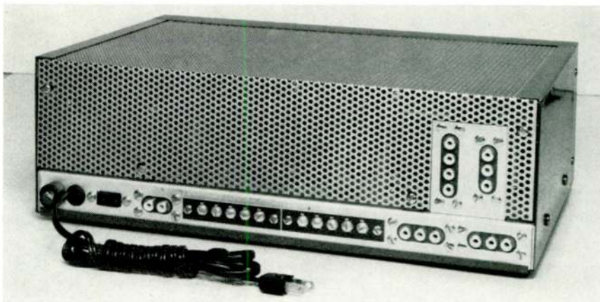
Fig. 8. There is ample ventilation for heat generated by the output tubes and rectifiers
