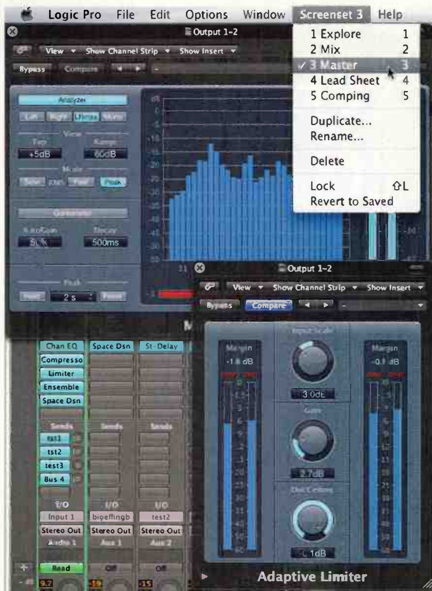
Figure 9. Logic's Screensets get their own menu for quick recall and switching among views.
