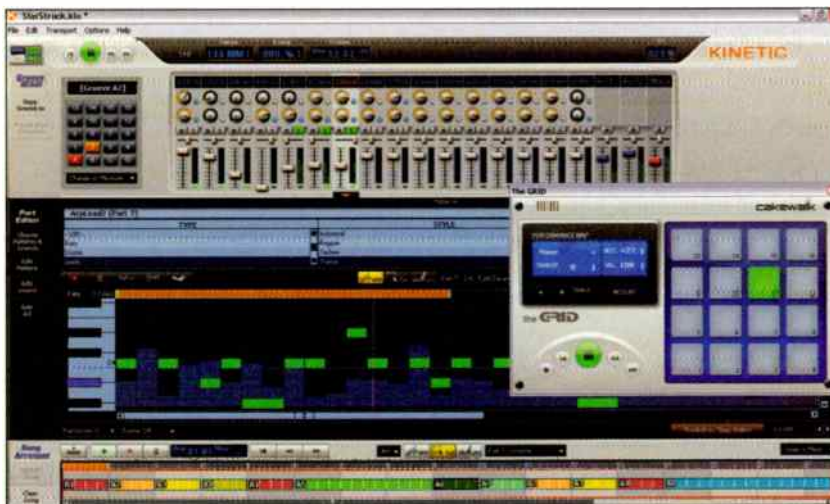
The top strip is the groove mixer, where each channel hosts a part. Note that the mixer settings can be totally different for each groove. Below that is the MIDI editor, and at the bottom, the song arranger. Toward the right is the Grid note entry interface, which can be triggered from a QWERTY keyboard.
