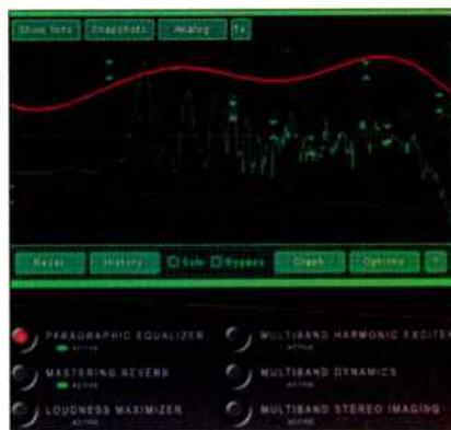
Fig. 2: iZotope’s Ozone 3 serves here as an accurate automatable EQ and reverb processor. All other FX are off. Note that the EQ curve is gentle, with no radical EQing.
