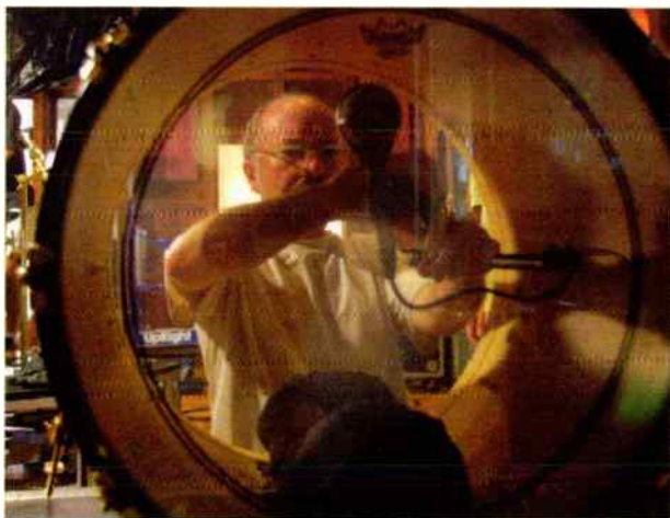
Recording Peart's closed-head kick was achieved via an adjustable mic-mounting device. "With a double-headed drum you'll want to get three inches from a head," comments engineer Paul Northfield. "The drum has enough natural resonance that you'll want a bit of closeness."
