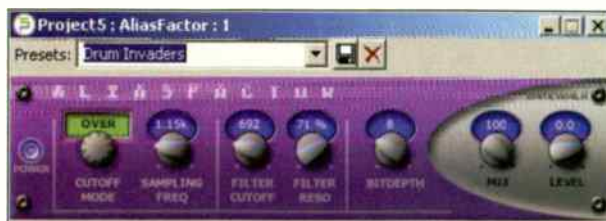
Fig. 3: Project5's "Aliasfactor" plug-in can change sampling rates and bit depth, but also throws in a filter too so you can mess up the frequency response.
