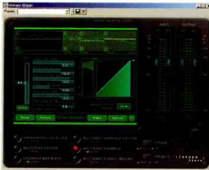
Fig. 2. iZotope's Ozone 3 is a "mastering suite" of processors that can also work well as a master bus effect. This shows the multiband compressor in action, but note that the loudness maximizer stage is also active to add a subtle amount of "brickwall" limiting.
