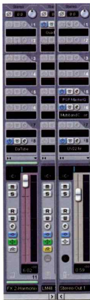
Fig. 1. This stereo output bus in Cubase SX is dedicated to mastering effects. The PSP MasterQ and a multiband compressor goes pre-fader, while the UV22HR dithering plug-in goes into the post-fader slot.
