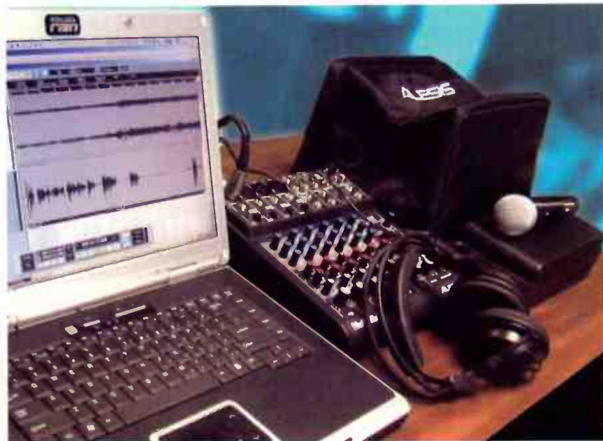
Fig. 1: The podcasting kit, set up and ready to go. The Rain Recording laptop on the left is running Cubase LE, with a track of music and another of narration. To its right are the MultiMix8 FireWire mixer, headphones, mic, mic case, and carrying bag. Not shown: desk mic stand.
