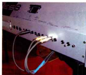
Loop cables over the arm of a keyboard stand to leave a little slack in case someone trips over a cable.
