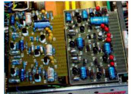
FIG. 4. NOTICE THE IDENTICAL COMPONENT LAYOUT, MAKING IT DIFFICULT TO DISTINGUISH NEW (LEFT) FROM OLD (RIGHT), EVEN WITH THE ORIGINAL CAPACITORS ON THE OLD BOARD, WHICH SHOULD BE CHANGED FOR BETTER PERFORMANCE.
