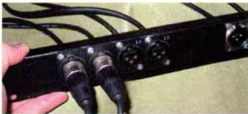
Fig. 3. I have a summing mixer (a Roll Music Folcrom), which is passive, and requires a mic preamp to bring the summed output signal up to line level. I built this XLR/preamp patchbay, allowing me to easily send a summed mix into a variety of preamps in my studio.
