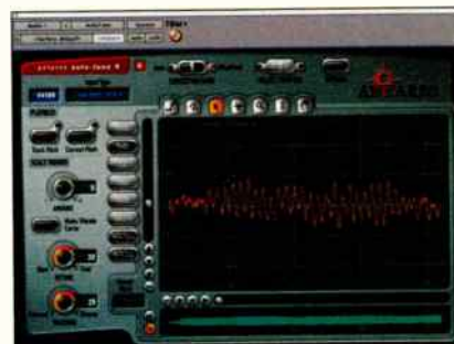
IN GRAPHIC EDITING MODE, AUTO-TUNE 4 CAN ANALYZE THE PITCH OF AUDIO ("TRACK PITCH"), AND DISPLAY IT GRAPHICALLY. THIS SCREENSHOT SHOWS A VOCAL NOTE WITH A VERY WIDE, SOMEWHAT ERRATIC VIBRATO.
