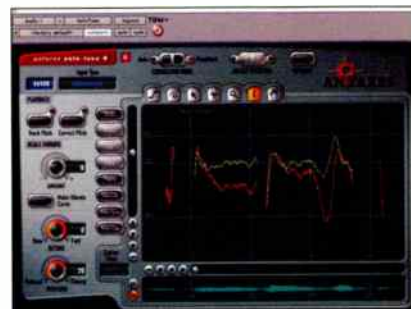
IN GRAPHICS MODE, THE RED LINE INDICATES THE TRACKED PITCH OF THE AUDIO. THE YELLOW LINE IS THE AUTOMATICALLY GENERATED CORRECTION AUTO-TUNE WILL APPLY. THE YELLOW LINE CAN BE EDITED USING THE TOOLS AT THE TOP OF THE GRAPH AND THE BUTTONS TO THE LEFT OF THE DISPLAY.
