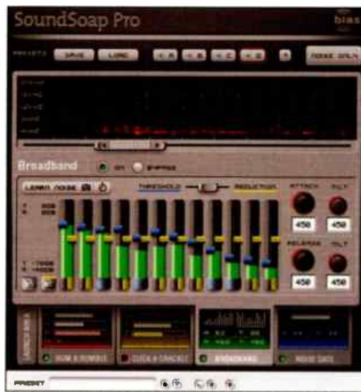
Fig. 3. BIAS SoundSoap Pro is a standalone program for the Mac designed to take a sample of noise, then subtract that from the audio signal. It also offers a other noise reduction tools, including noise gating.
