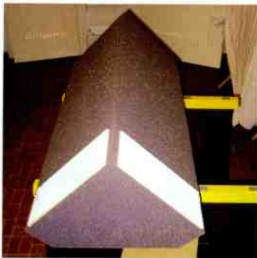
I HUNG THE BASS TRAPS (SHOWN HERE) FROM RING HANGERS ATTACHED TO PIECES OF 1/4" BOARD GLUED TO THE BACK.
