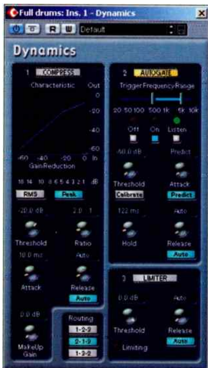
Fig. 1. The Autogate section of Cubase SX 2's Dynamics module includes all of the traditional functions, but also offers gating based on frequency so that only particular frequencies open the gate. This makes it useful as a special effect as well as for reducing noise.
