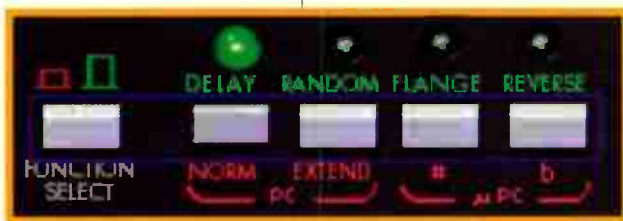
THE H949 CAN OPERATE IN ONE OF SEVERAL MODES, INCLUDING PITCH SHIFTING, DELAY, FLANGE, AND REVERSE, WHICH LETS YOU CAPTURE A 400 MS PIECE OF AUDIO AND PLAY IT BACK IN REVERSE.
