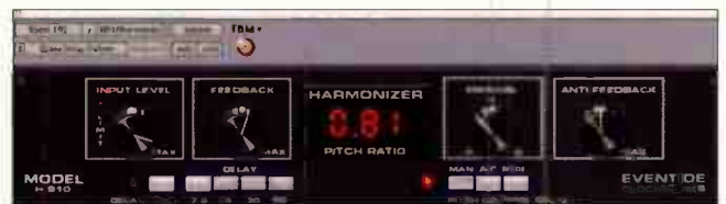
ONE OF THE FIRST DIGITAL EFFECTS ON THE MARKET THE ORIGINAL H910 HARMONIZER COULD SHIFT PITCH UP TO ONE OCTAVE UP OR DOWN AND HAD A BUILT-IN DIGITAL DELAY.
