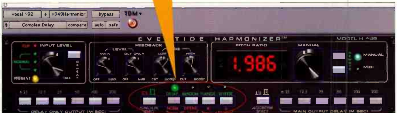
THE H949 HARMONIZER WAS ONE OF THE FIRST MULTI-EFFECTS BOXES AVAILABLE, OFFERING THREE OCTAVES OF PITCH SHIFT, DELAY, FLANGE, AND A REVERSE MODE.
