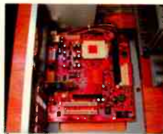
Fig. 8 Completing the motherboard installation. After screwing the motherboard into the standoff centers, attach the power supply,
