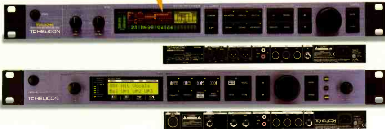
THE DISPLAY ON THE VOICEONE PROVIDES PLENTY OF USEFUL INFO ABOUT THE INCOMING SIGNAL'S PITCH, AS WELL AS THE PITCHSHIFT KEY, AND MORE.
