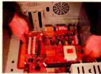
Fig. 7 Make sure the ports will fit through the holes in the back of the case by placing the motherboard on the standoffs.
