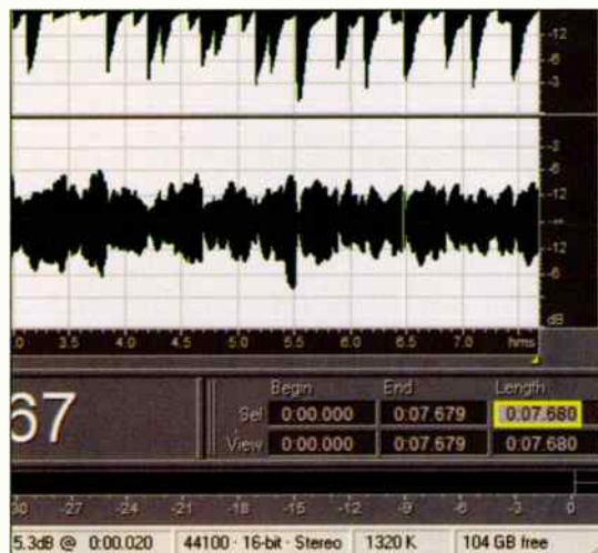
In Cool Edit Pro, simply typing a new value into the Length field (outlined in yellow for clarity) can trim a file to a specific number of samples.
