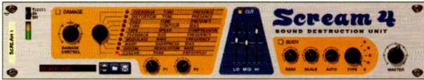
SCREAM 4 SOUND DESTRUCTION UNIT — RUDE AND ROCKIN'; THIS UNIT HAS JUST THE RIGHT COMBINATION OF TOOLS FOR SERIOUS SONIC SHREDDING. CHOOSE THE "DESTRUCTION" TYPE FROM THE DAMAGE SECTION, THEN SCOOP OR PUSH THE LOWS, MIDS, OR HIGHS WITH CUT. FOR HYPER FILTER RESONANCE SOUNDS, TURN ON BODY AND START TWISTING KNOBS.
