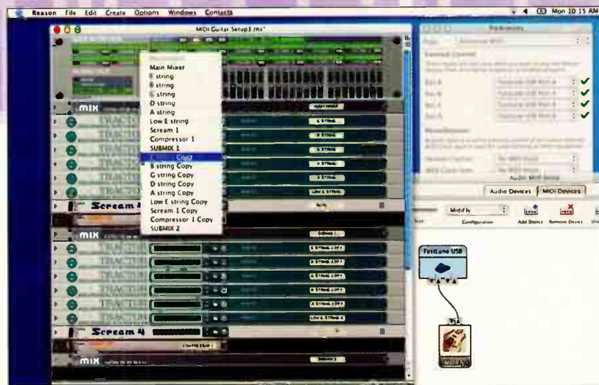
HERE'S THE ACTUAL SETUP JERRY HAS USED ON SEVERAL SESSIONS, WITH TWO SUBTRACTORS PER STRING, DISTORTION, AND COMPRESSION. THIS SCREENSHOT SHOWS THE HIGH E STRING BEING ASSIGNED TO A SUBTRACTOR THAT RECEIVES ITS INPUT FROM MIDI BUS B.
