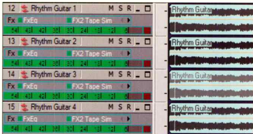
HERE A GUITAR TRACK HAS BEEN "CLONED" THREE EXTRA TIMES IN SONAR, WITH EACH INSTANCE FEEDING AN EQ AND DISTORTION PLUG-IN. THESE HAVE BEEN ADJUSTED, ALONG WITH PANNING, TO CREATE MULTI-BAND DISTORTION.
