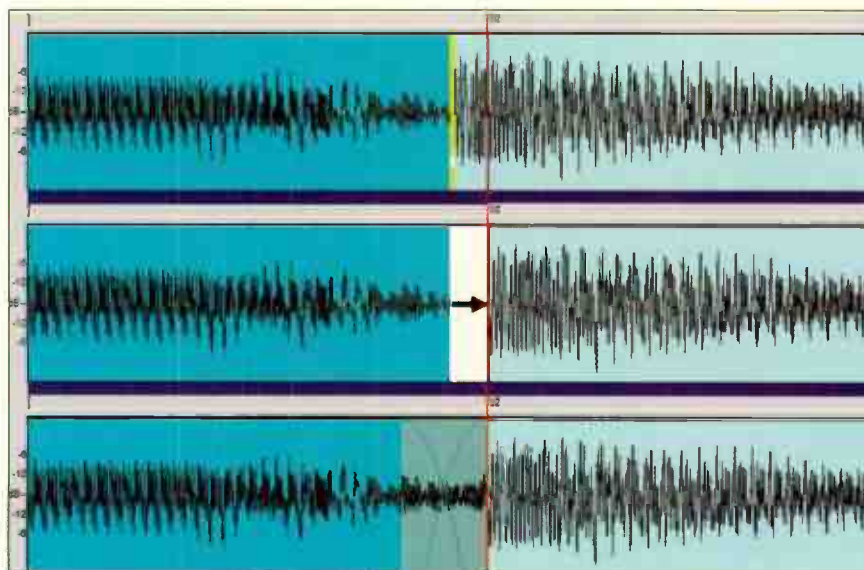
FIG. 4. THREE STEPS INVOLVED IN QUANTIZING A NOTE THAT LEADS THE BEAT.
