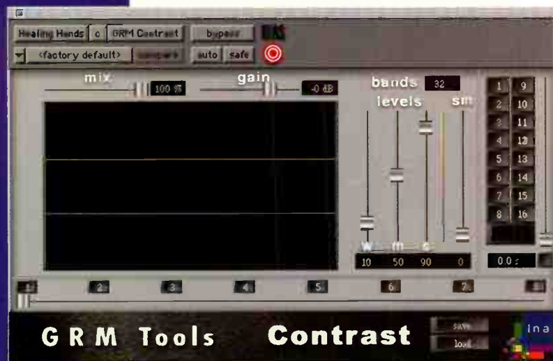
Contrast lets you independently change the gain of low, medium, and high volume frequencies that comprises a signal.
