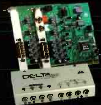
DELTA 66 & DELTA 44 - 24 bit/ 96 kHz full-duplex recording interfaces.
