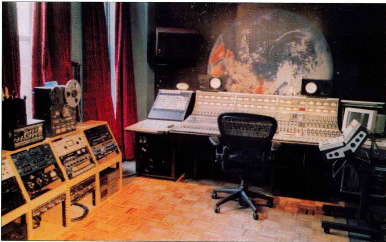
MISSION CONTROL ROOM: A vintage 32-channel Neve 8068 was a major acquisition for the analog/digital hybrid studio.
