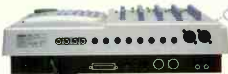
The back panel of the FD-4 shows off its tremendous flexibility. Balanced XLR Mic inputs, optical S/PDIF and MIDI in and out, SCSI-II plus standard analog ins and outs make the FD-4 adaptable to any application.
