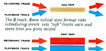
The ADAT format records each track discretely, as all professional multitrack recorders should.
