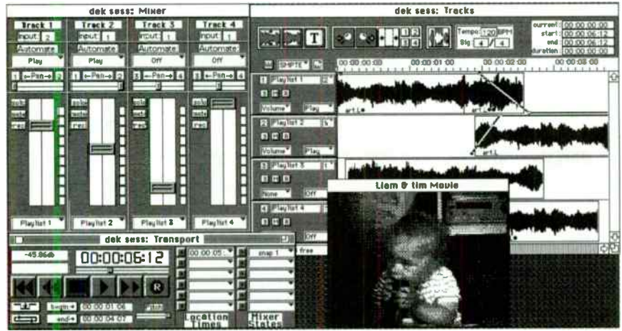
Figure 5: Deck 2.0 not only offers comprehensive recording, editing and mixing features, it can also function as an all-digital post production studio for QuickTime movies.
