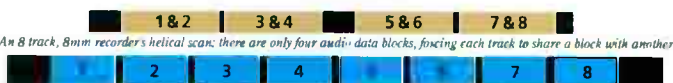
An ADAT's helical scan: ADAT tracks are safely separated into 8 discrete data blocks. (Both vertical dimensions enlarged for clarity)
