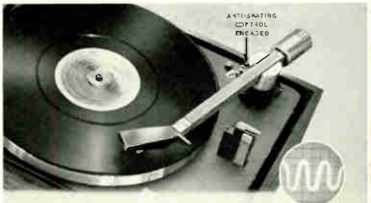
5 "Now watch me neutralize the skating force. I swing the anti-skating control back into position... and the arm tracks as perfectly as if there were a groove in the record! If I were playing a regular record—with the side pressure gone and resulting distortion eliminated—the sound would be cleaner."
