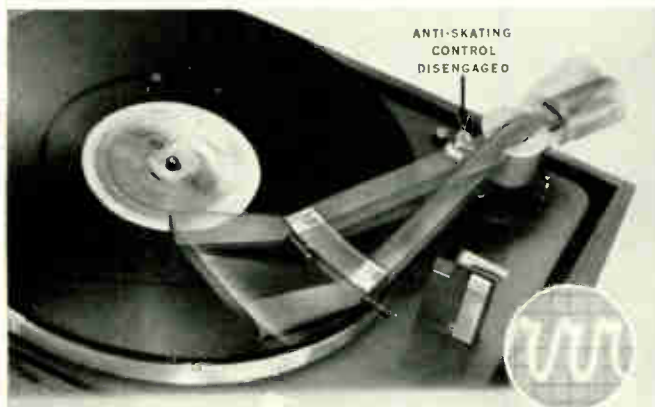
4 "Now you can actually watch the strength of the skating force. I start the Lab 80, but flip the anti-skating control over and out of operation. Note that as soon as I put the stylus on the grooveless record, the arm moves rapidly... with force, toward the center."
