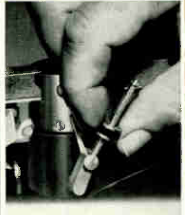
3 "I then slide the counterweight on the anti-skating control to the second notch... equivalent to the tracking force I have just set on the tone arm."
