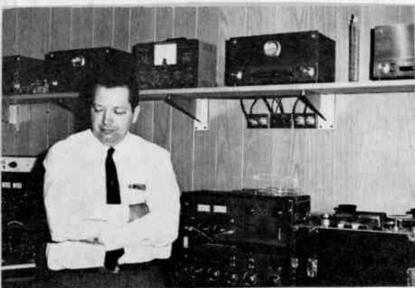
Four 70 watt mono power amplifiers are mounted openly on a shelf to assure good air circulation. Note the audio wall jack outlets under the shelf—mark of an audio hobbyist.
