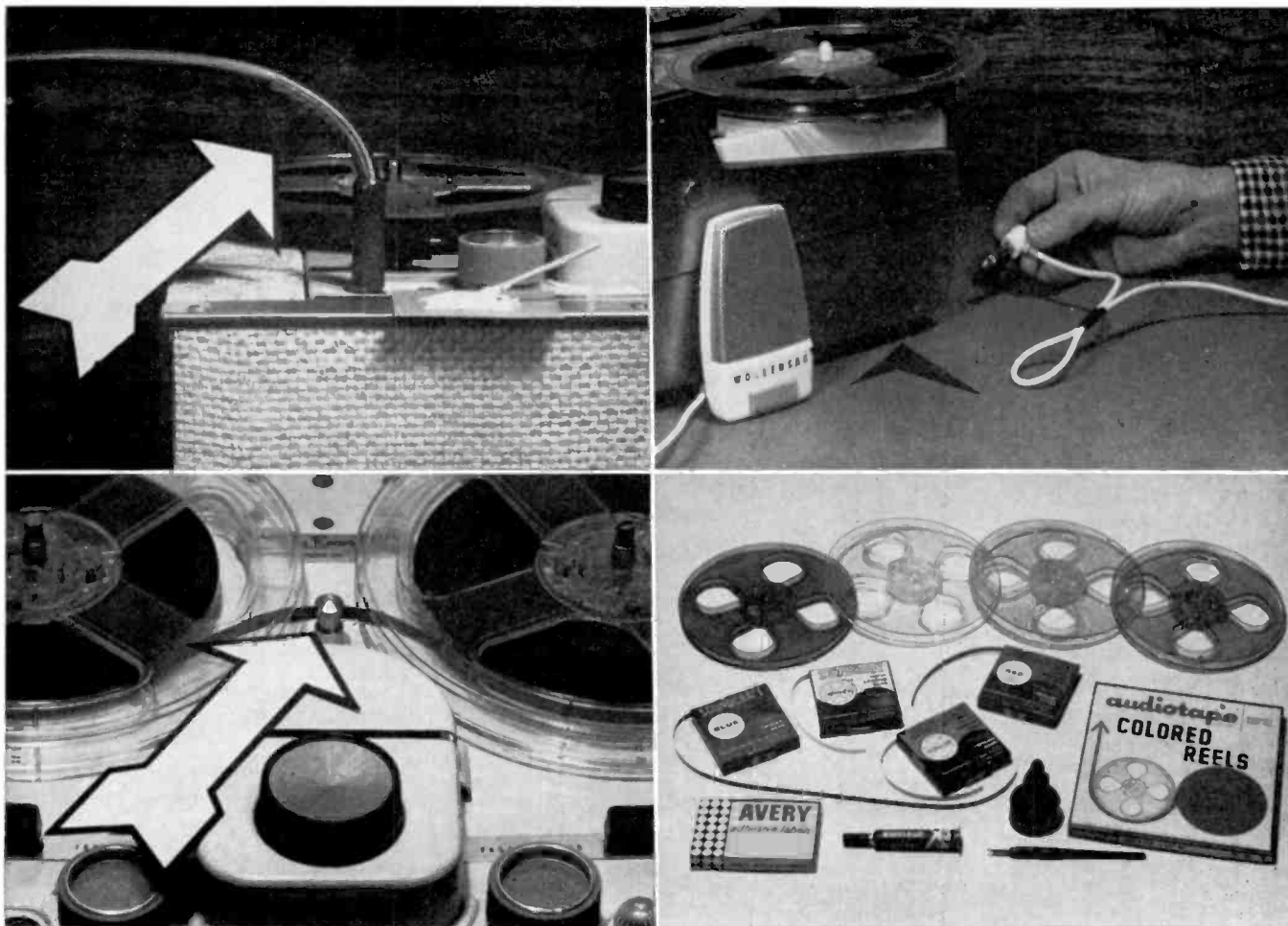
Fig. 2 (upper left). It's a sad occasion when a microphone "goes dead" suddenly, as always, without a bit of warning. So since it's the PLUG that gets the most abuse, I relieve the strain quite a bit by adding a small spring over the end of the cable that goes inside the plug, and I fill the plug itself with gobs of heavy-consistency Epoxy. Fig. 3 (upper right). Another sure-fire way of avoiding strain on mike (and other) cable plugs attached to your recorder, is to form a SMALL LOOP in the cable itself, about ten inches or so from the plug end. Plastic tape will hold this loop securely. Then, whenever you plug in the cable, anchor this loop under one "foot" of the recorder. Fig. 4 (lower left). With my recorders that don't have automatic tape lifters, I try to cut down on extra head wear whenever I have to race a reel of tape from one side to another, by by-passing the heads completely. This works fine except that the wind-up is then rather sloppy, unless you install an AUXILIARY TAPE GUIDE between the reels. Fig. 5 (lower right). Here are some of my favorite recording accessories. Until I switched to using COLORED REELS and COLORED LEADERS I was having a terrible time keeping the different types and thicknesses of tape separate. Now, along with adhesive labels and even special marking inks to also aid me, my tapes are automatically identified.
