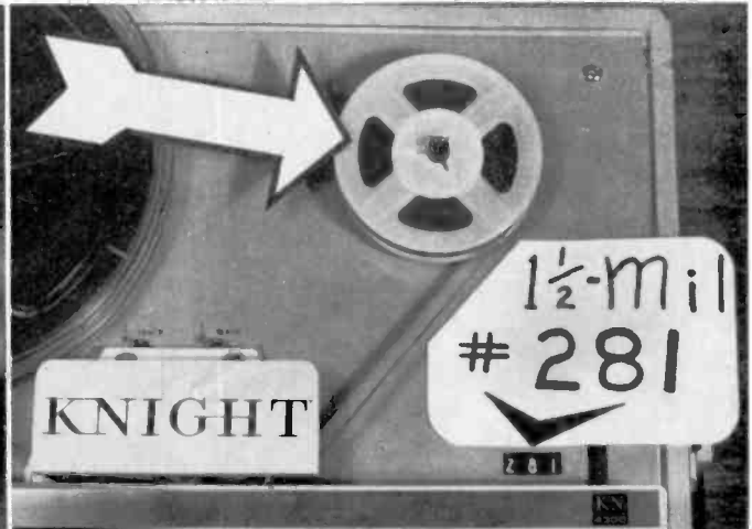
Fig. 6 (upper left). Both the plastic reels (which come in 5" and 7" sizes) and the Mylar leaders come in four colors: blue, yellow-gold, red and green. There's also a white leader to go with the clear reels. And with these new WRITE-ON-ANYTHING FELT PENS being sold everywhere now, it's a snap to write directly on the leader tape. Fig 7 (upper right). After lots of use, some plastic tape reels become a bit sloppy around the hub. They've been put on and taken off so often the center hole has become enlarged to the point where the reel fits on the spindle in a rather loose and wobbly way, finally affecting tape movement. A set of REEL LOCKS will correct this. Fig. 8 (lower left). If you have an unmarked reel or portion of a reel of tape, it's difficult to know how long it will run without slow-running it through your recorder to find out. A much quicker way to find out is to run it on FAST FORWARD through your machine, then compare the seconds elapsed to a previously made correlated table. Fig. 9 (lower right). Ever pick up an old reel of unidentifiable recording tape and wonder WHAT THICKNESS TAPE it was? You can make a quick check in no time flat by fast-forward running the tape onto a 3" reel. Starting with the index counter at "000," I know immediately by the time the reel is full just what thickness the tape has to be.
