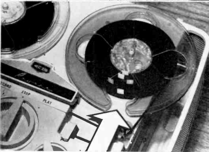
Fig. 10 (upper left). For those of you who do a lot of editing, here's a handy way to set your index counter TO A CERTAIN NUMBER (not just back to zero) when the occasion warrants. Hook a 3" reel and a large-hub 7" reel up as shown here, then run your tape recorder on fast forward or fast rewind until you reach the number you want. Fig. 11 (upper right). Ever hear of REVERSED index numbers? On monaurally recorded 4-track tape it takes time to locate a certain passage on the 2nd or 4th track because you first have to run the tape all the way from one end to the other, so the index numbers will work out. Unless, of course, these tracks are indexed in reverse (see text). Fig. 12 (lower left). Reverse-indexing is a bit of a chore, but once it's accomplished for a particular 4-track reel of recorded tape, it's pure pleasure finding ANY passage, no matter on which track. To aid you in backing up to the 2nd and 4th track positions, you can use either an "open-faced" reel or a "cut-into" reel as shown here. Fig. 13 (lower right). If you're like I am about recorder troubles, you pretty well ignore them until they actually come a-knocking. But since they surely will, here's one LAZY MAN'S APPROACH to foreseeing and forestalling a few of them, along with some other helpful hints.
