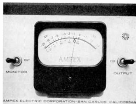
Above: When adjusting an alignment tape in a machine, care should be taken to reach the point of maximum output for the reproduce head, since a lesser peak will occur on each side of the maximum output position.
