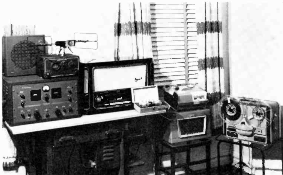
The writer's equipment. Left to right: Hammarlund super-pro shortwave receiver; on top of that, the speaker, a Panadaptor (to examine the incoming signal visually) and a directional FM antenna; the Telefunken FM-AM receiver; the Fi-Cord transistorized recorder; the Wollensak atop the Revere; the Revox with 10" reels and built-in fader-mixer.
