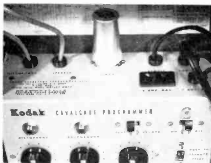
Connections are grouped in well of Programmer. Two grey wires at left go to recorder microphone and external speaker jacks, two black wires at right to projector power supply and remote control. Other lead is power supply.
