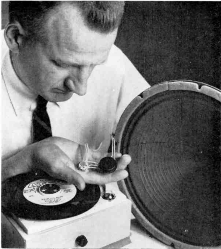
Above: an example of micro-miniaturization is this Westinghouse developed molecular electronic function block being used as an audio amplifier in a conventional system. Frequency range is 0 to 20,000 cycles and output is 5 watts. Amplifier itself (at right in black mounting) is tiny device whose volume is .001 cubic inch. Device at left is molecular electronic preamp. Upper right: Old type tube, modern tube and transistors showing relative size reduction. Lower right: standard transformer, small object on top is transistor transformer.
