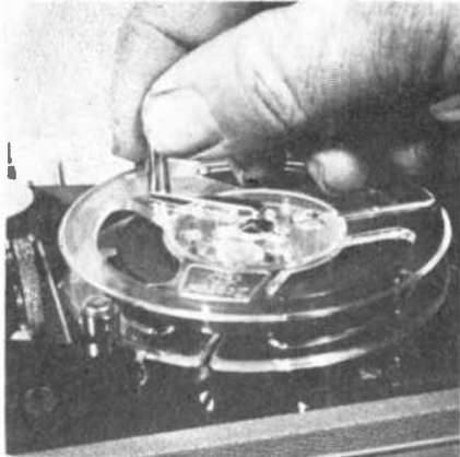
Rewind can be done by hand, to save battery drain, by inserting handle furnished in one of the slots on the reel and turning it. Handle is stowed alongside batteries.
