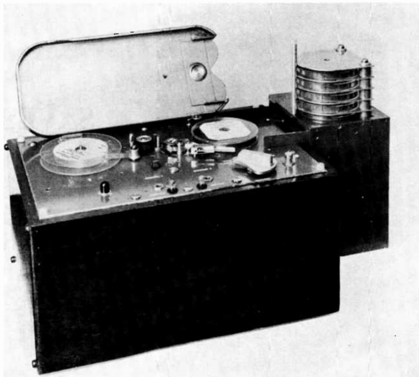
Armour Research Foundation cartridge machine with top raised to show mechanism. Unit uses \frac{1}{4} inch tape on reel-type spool and is said to be compatible with present day recorders.
