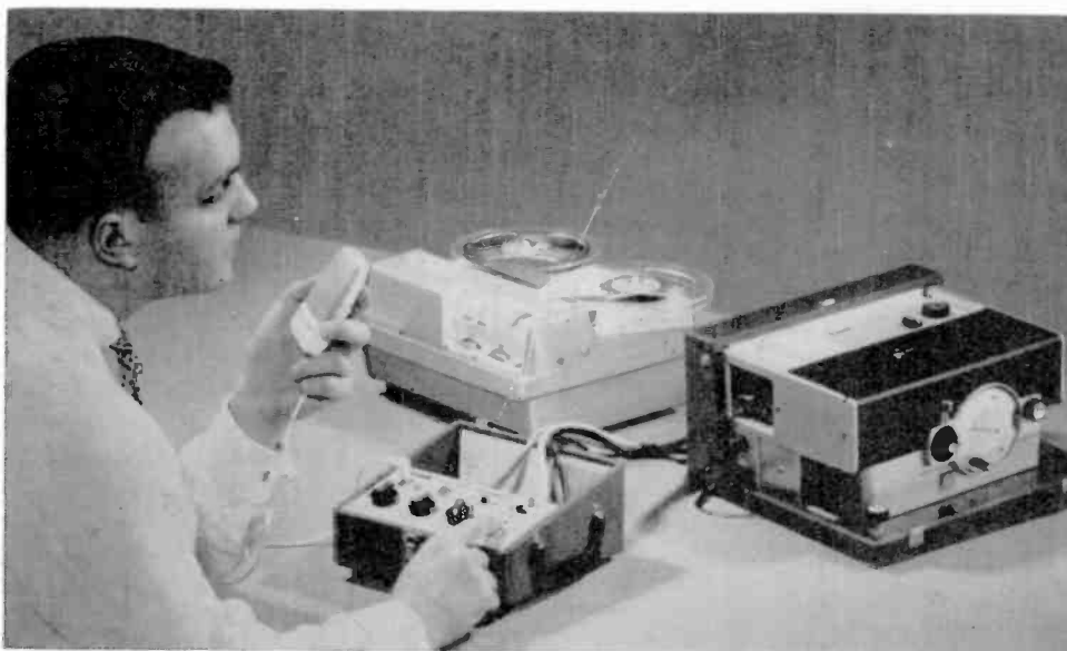
There are an increasing number of devices coming on the market which will enable the tape recorder to operate the projector from signals placed on the tape. Shown is the new Kodak Programmer and Calvacade automatic projector. Both slides and tapes should be edited carefully for maximum viewer interest.
