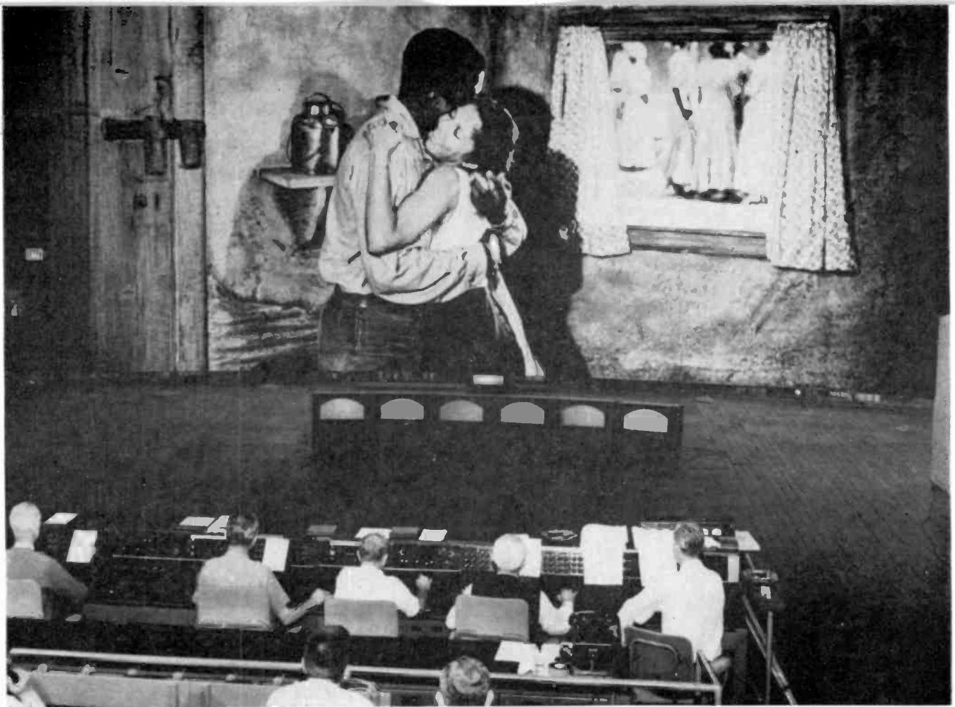
"Bess, You is Mah Woman Now," sings Porgy (Sidney Poitier, mouthing the voice of Robert McFerrin) to Dorothy Dandridge while Todd-AO technicians "mix" music, dialogue and effects, "swinging" the six sound tracks to follow the action across the screen. Six VU meters in front of curved screen register sound levels of each track. Counter above meters keeps tab of film footage.
