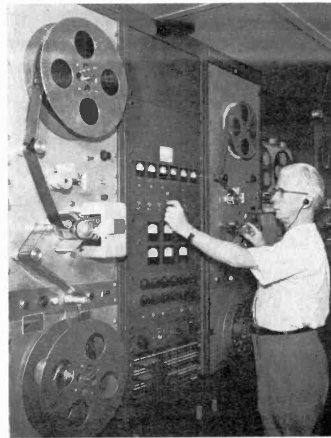
Eyeballing levels of sound on VU meters, machine operator uses ear plugs to listen in while recording from six-track 35mm magnetic sound film (right) to six tracks of 70mm picture film (left).
