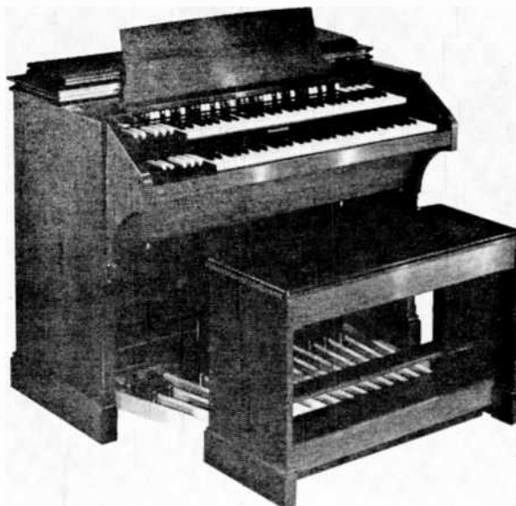
The large console type Hammond organ may have integral speakers or a separate tone cabinet. Recording takeoff can be made at pre-amplifier. Output voltage at speakers may go as high as 10 volts.
