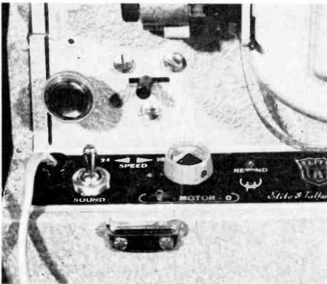
Left side of recorder control panel showing amplifier on-off switch, speed shift lever, function control (motor and lamp on and off) and rewind button which is depressed to rewind.
