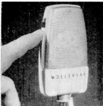
Upper: Left side of recorder showing cutoff switch, speed control, odometer counter, record and overload indicators. Center: right side showing automatic reversal contact, tone and volume controls and record and play buttons. Lower: bar lifts out for access to heads for cleaning. Below: button on mike controls recorder.
