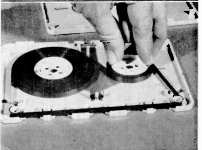
Should a break occur in a tape cartridge, pull out enough tape to provide working room. Overlap ends and cut through both at an angle with scissors. Apply splicing tape to shiny side of tape and then replace tape in the guides. Tighten by turning take-up hub and replace cover.
