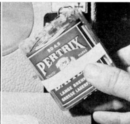
Back of case opened to show placement of batteries and speed shifting control. Batteries are standard 4 1/2 volt and fit in plastic holders which slide in the wells provided as shown. Back of recorder swings out to give access to batteries and speed shift.
