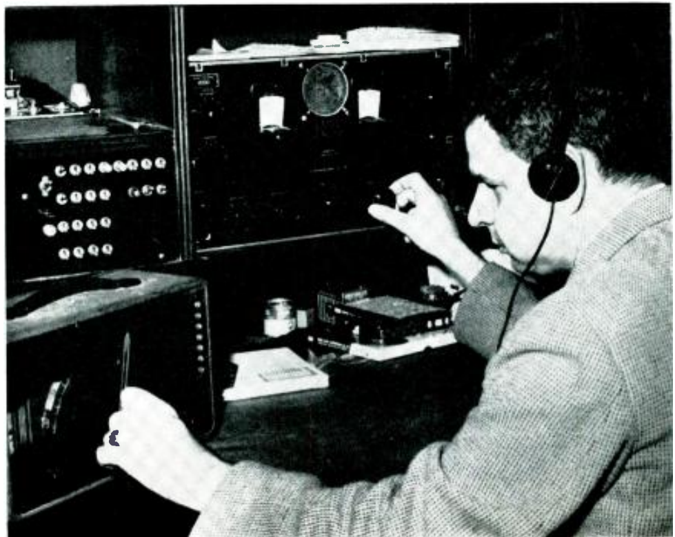
Professor Thomas A. Benham at the radio and recording gear he used to record all satellites through Explorer III. The Russian Sputniks broadcast on 20 and 40 megacycles, the American satellites on 108 megacycles. Professor Benham is totally blind.
