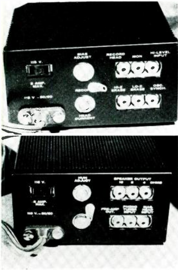
Upper left: rear of Nortronics RA-100 record amplifier. Connections include 110 v. AC outlet, Bias adjustment, Recording head input, Mon input, Hi-level input, Head current, High and low impedance erase outputs and Oscillator Synch. Lower: rear of PL-100 playback. Connections are: 110 v. AC outlet, Hum adjustment, 16, 8 and 4 ohm speaker outputs, Pre-amp output, Phono or tuner input and Magnetic head input. Right, upper: drawing shows connections from Stereo Kit to amplifiers. Lower: one channel of the head may be connected to the recorder if a jack is used to disconnect the recorder head. This permits use of the recorder as one side of a stereo system.
