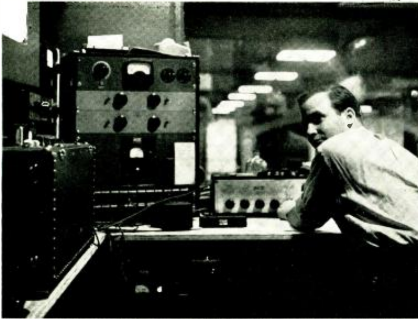
A study of an engineer at work. Steve Temmer watching the meters of the two Ampex recorders while mixing the mike lines to get the best stereo balance.
