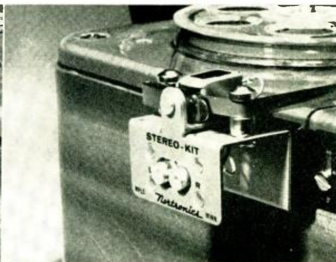
must travel accurately through the guides. Head position is adjusted by moving the bracket as necessary. The recorder is used simply as a tape transport.
