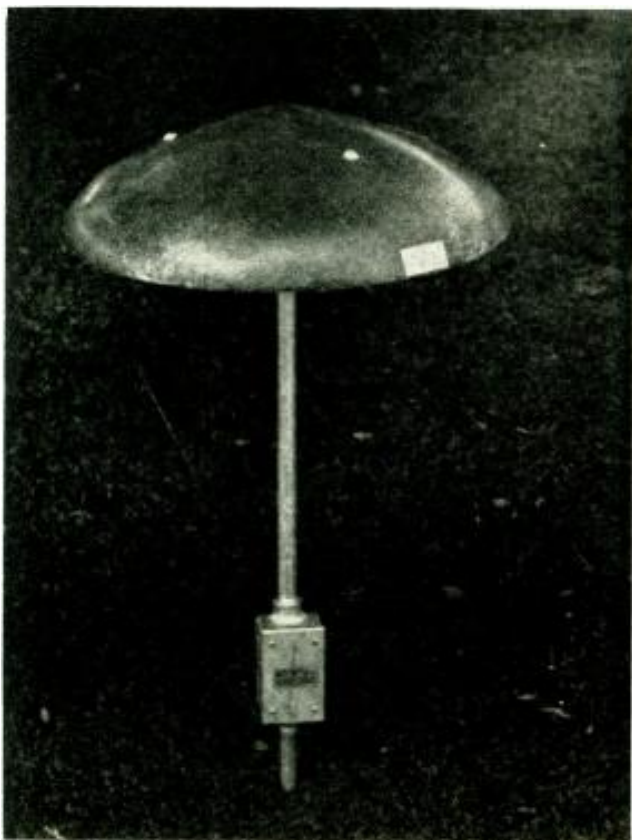
Permanently mounted garden speaker. Outlet box shaft extends into ground to hold speaker upright. Buried waterproof cable is run underground to speaker location.
