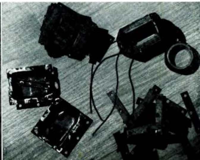
All you need to get started on making a bulk eraser for tape is an old power transformer which can be obtained from your own junk box or from a radio or TV dealer. The primary winding must still be in good condition, the secondary does not matter. Take it apart as explained in the text and save the coil and the "E" laminations (upper left of photo).
