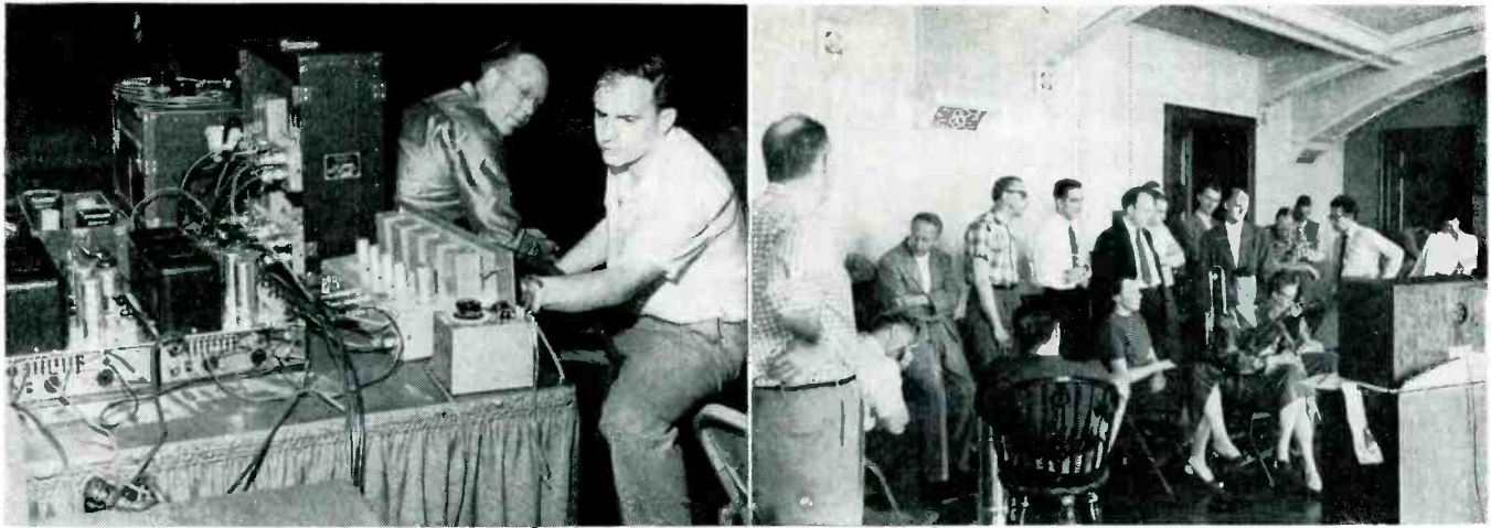
Left: the author adjusting microphone levels for a two channel recording. He maintains that with proper placement of mikes and arrangement of musicians, two mike channels produce more realistic recordings than multi-mike pickups. Right: vocalists and musicians taking part in the recording session listening to the playback.
