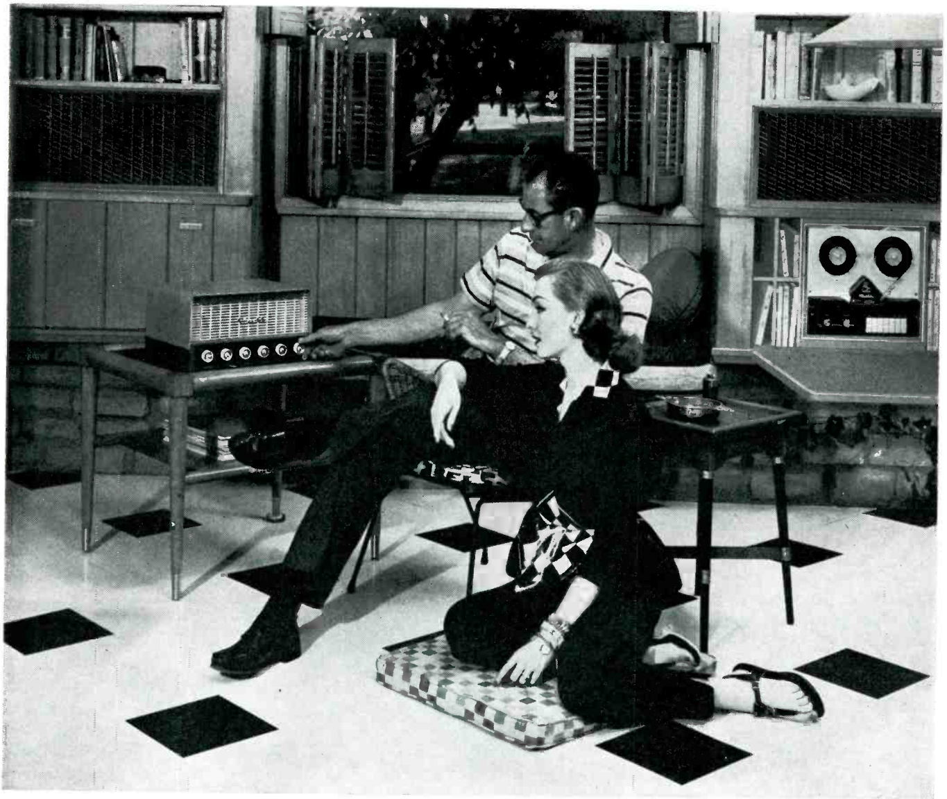
Stereo sound has brought living music to the home. Shown above is a system which uses a tape transport mechanism, or deck, on the right to feed a dual channel amplifier, center. The output from the amplifier is fed to the two speakers built into the room. Transport and amplifier are by Bell Sound Systems.
