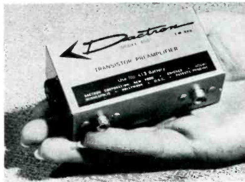
Upper left: the drawing shows how a small Telex type jack is installed in the head cover and connected so that when the jack is inserted the recorder head is disconnected and the current from the Steradapter fed to the amplifier. Lower left: the transistor pre-amplifier which may be used with the Steradapter. Above, three ways of making the connections for stereo sound.
