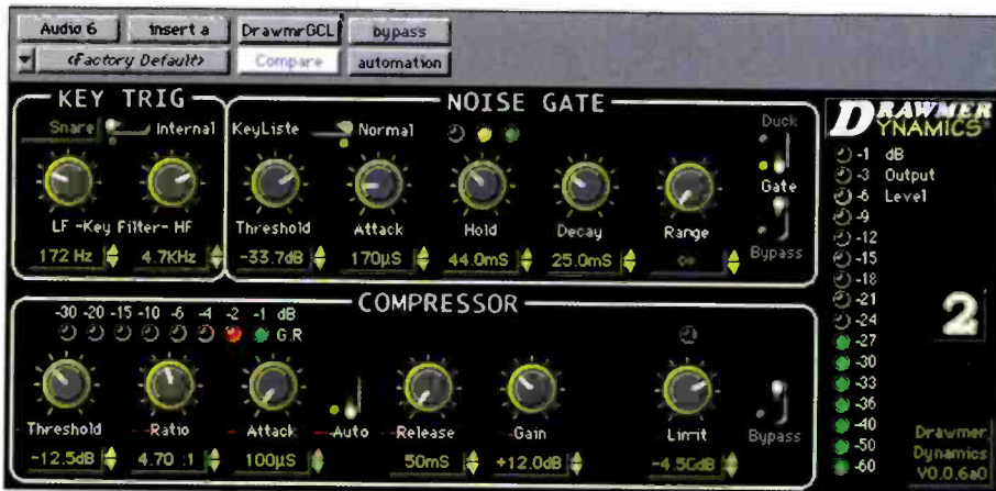
Drawmer Dynamics plug-in with two alternative sets of dynamics processing
