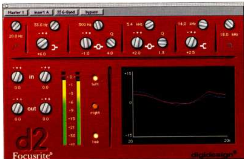
Focusrite's d2 with up to six bands of EQ
