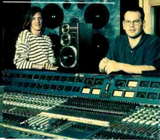
Power plant 78-input GML-Neve 8048 console built between April 1988 and April 1989. Designed by Nicholas Clarke and Clifford Brown
