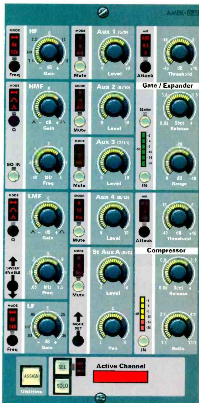
Panel detail—EQ, auxes and dynamics under assignable control
