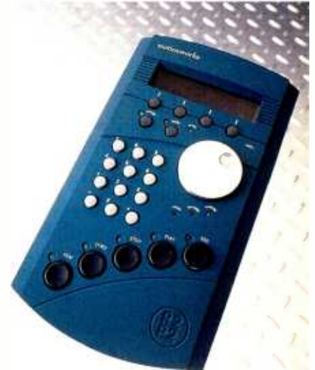
The Motionworks R2P2 remote controller opened with a library of 140 machine profiles—with more to follow
