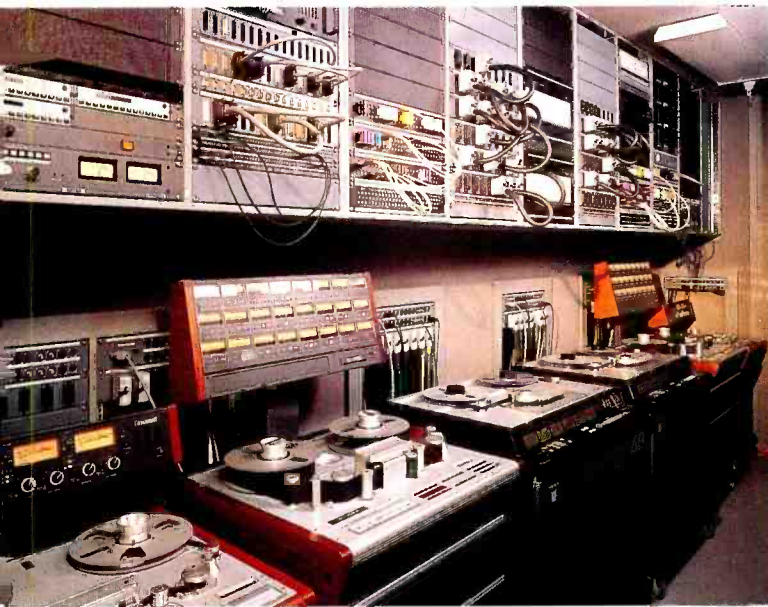
Sony 3348s, Studer 827 and 820 machines in the common equipment room. Note the comprehensive patching arrangements above the machine bay
