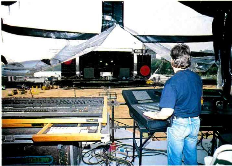
With each band using its own consoles and control equipment the channels required to run the PA ran to in excess of 600
