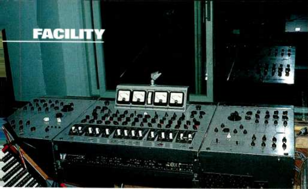
Lenny Kravitz' valve console: the EMI Redd 37
