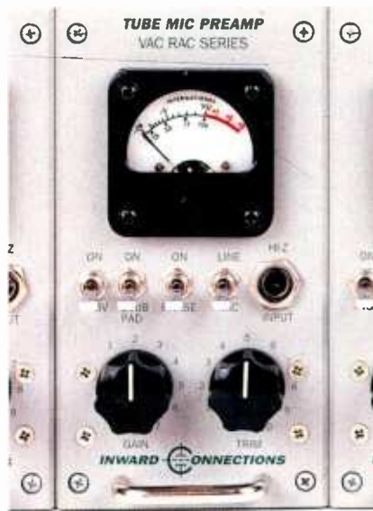
The Vac Rac's mic preamp module
