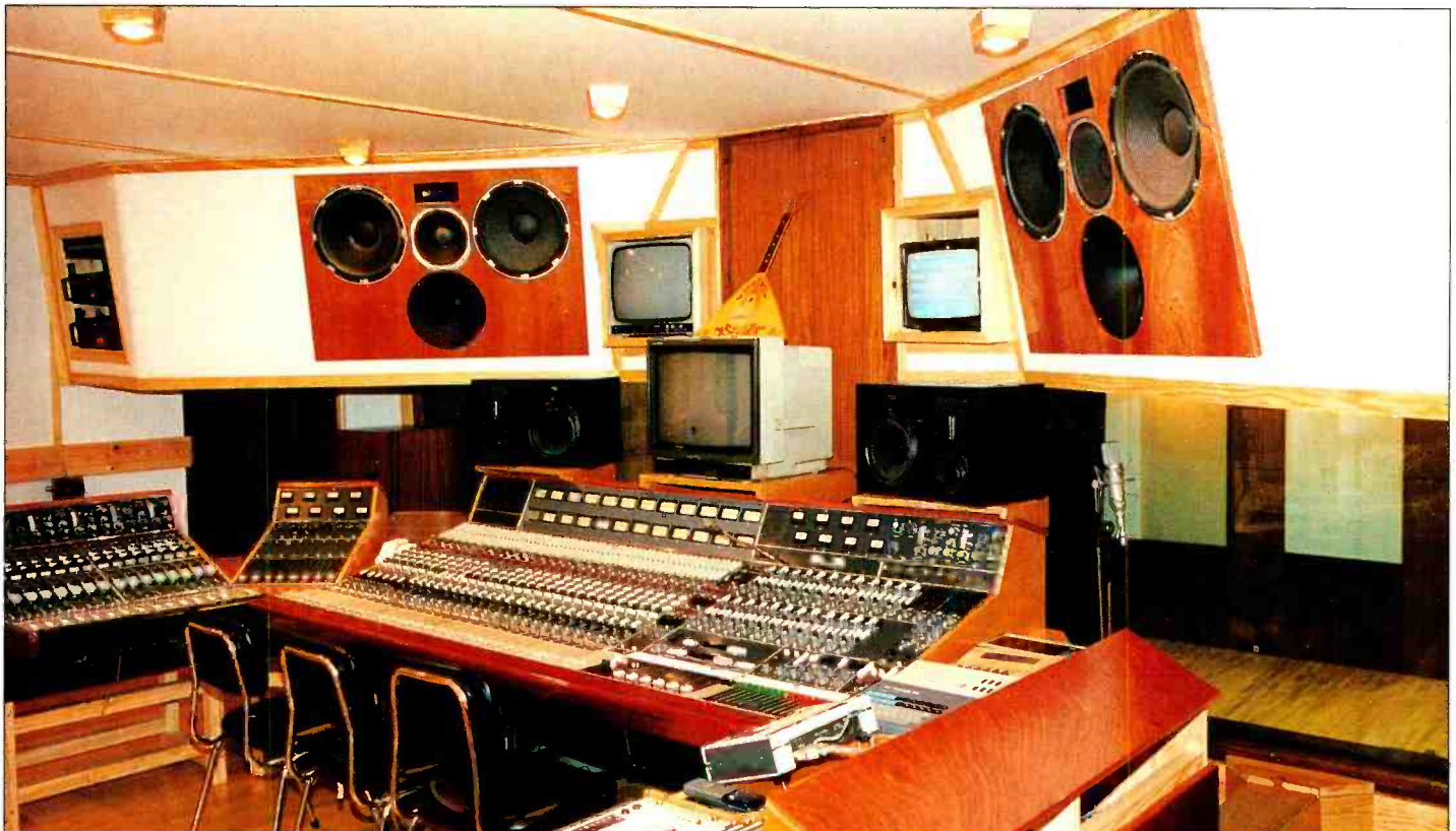
The redesigned studio control room with Reflexion Arts 236 monitors and 'combined' Neve console
